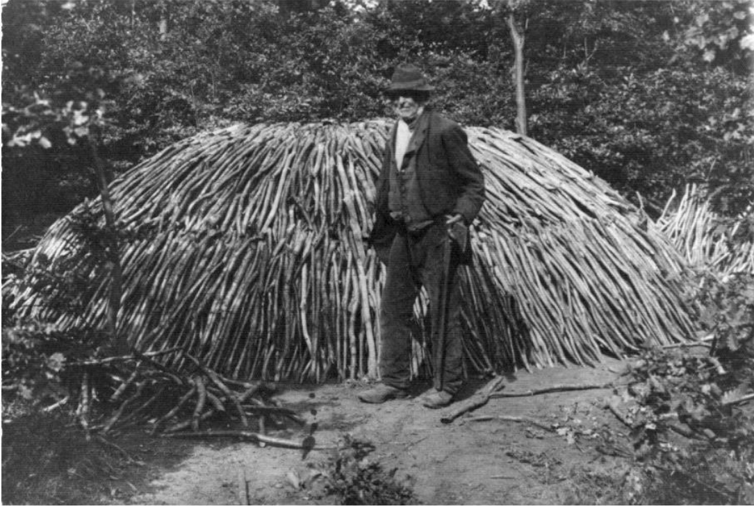
A charcoal heap prior to covering and burning - Wyre Forest late 19th Century
